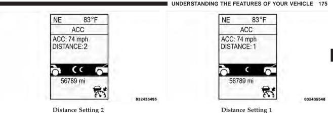
To change the distance setting, press the Distance button and release. Each time the button is pressed, the distance setting adjusts between long, medium, and short.
